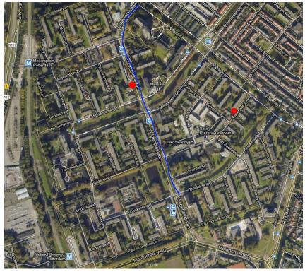
Figure 1: Locations for noise measurements along the Wilgenplaslaan and Teldersweg in Rotterdam. The blue marked road will be repayed with reduced noise layer.
