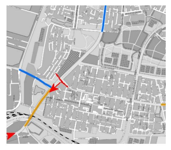
Figure 2: QUADMAP pilot area Groene Kruisweg; blue marked road will have low noise pavement in 2013 and orange marked roads were repayed in 2011 and 2012
